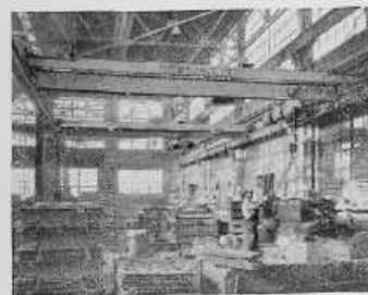
Single I-Beam Cranes carrying floor operated Shepard Hoists. Serves every purpose of a crane.
